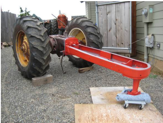
Moving tractor for overall painting. Note dolly in place of missing front wheels.
