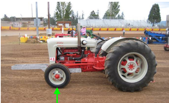
More weight on front wheels than Oliver 66, but similar weight balance.
