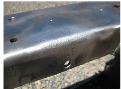
Ground and ready for primer
