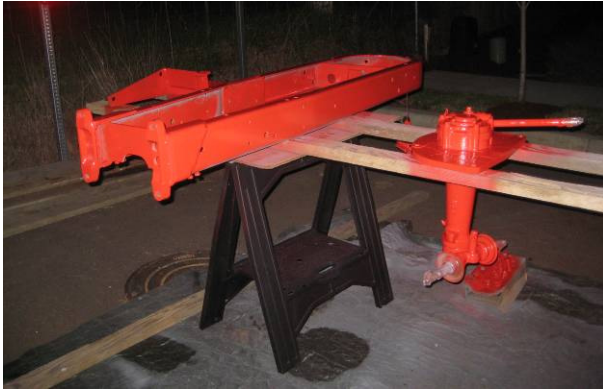
Painted frame and front pedestal
