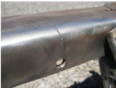
Original crack (bottom of frame)
