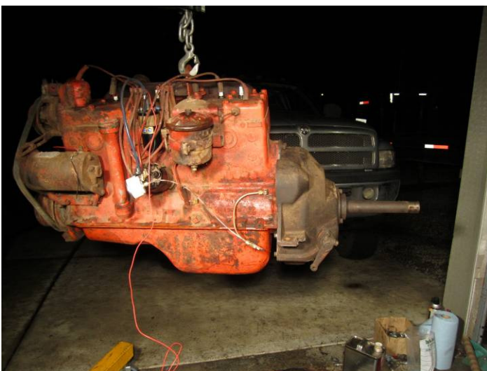
The 265 with bell housing installed
