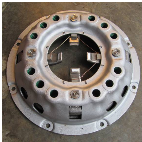
The same pressure plate after rebuild
