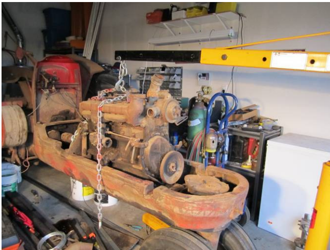
Lifting out the Chrysler 201
