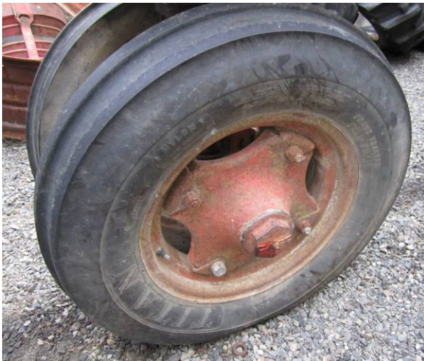
Heavy cast front wheels
