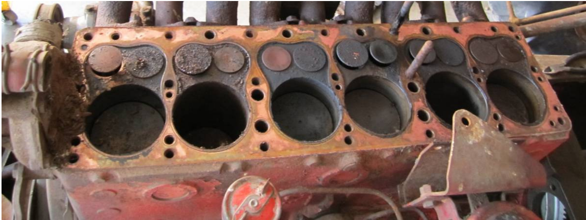
Head removed, exhaust valve on #1 and #4 are stuck
