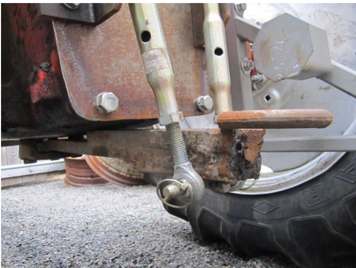
Original drawbar used that had other pieces of metal welded to it in the past.
