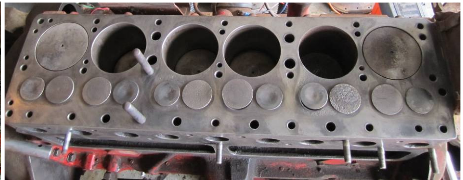
Valves unstuck, lapped, & everything cleaned. Absolutely no ridge in the cylinder walls. Gotta love a low hour combine engine!
