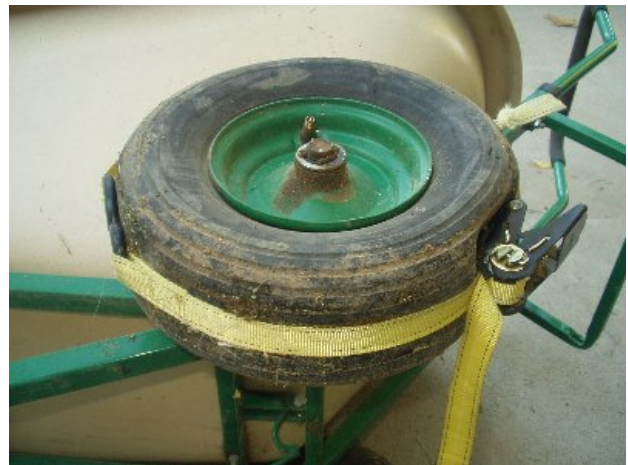
This example shows how to run the strap around the tire when inflating
