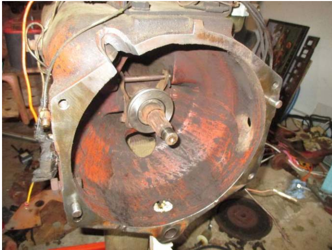
Bell housing cleaned and new release bearing installed
