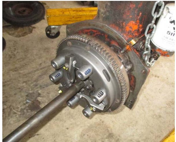
Clutch installed, notice CA shaft used to align disc with pilot bushing
