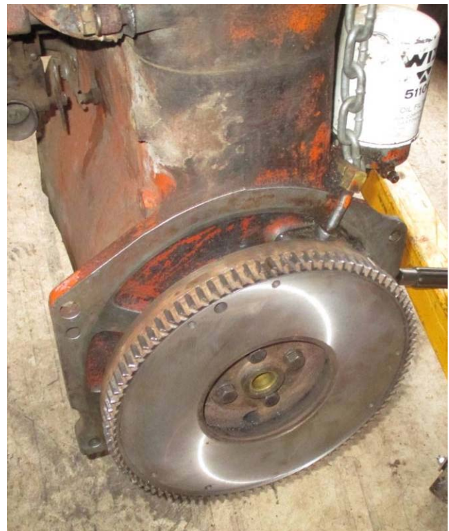
Surfaced flywheel installed
