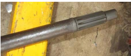
Allis CA drive shaft to use as a clutch alignment tool
