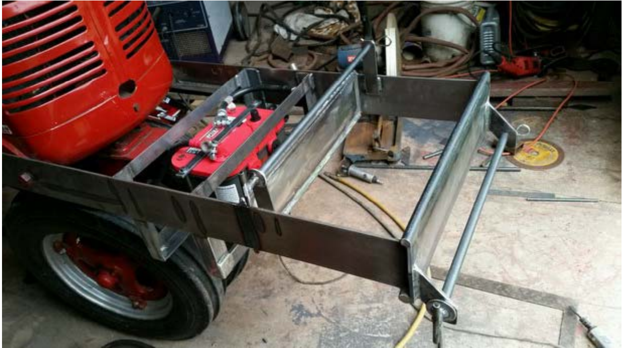
This view shows the added tabs with cross bars to keep weights secure.
