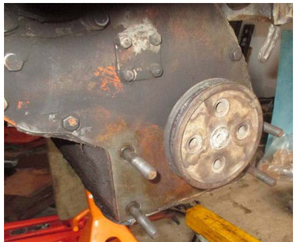
Studs installed into front of engine block
