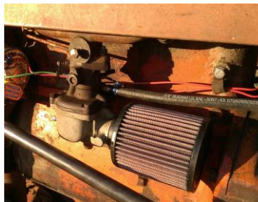
Farmall 706 Carburetor and K&N filter
