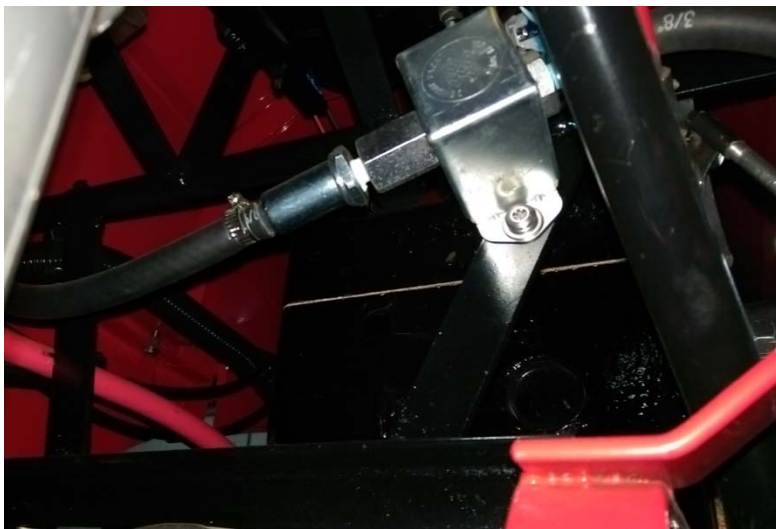
Fuel pump installed to fuel tank lattice
