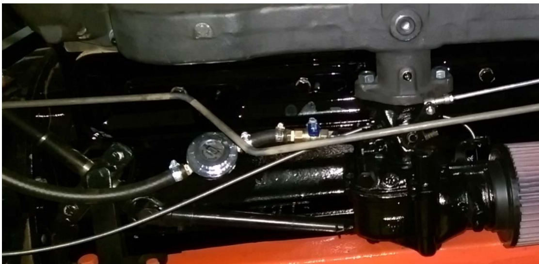
Note round fuel pressure regulator mounted inline, also ¼ turn ball valve fuel shut off at carb
