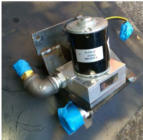
Water pump ready for paint
