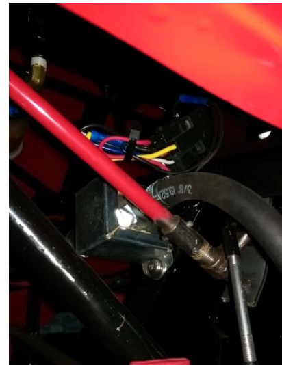
Fuel line to carburetor, throttle linkage in foreground
