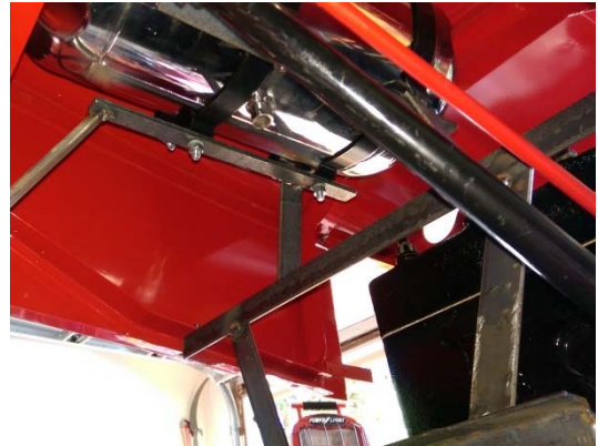
Fuel tank in position with some bracing added
